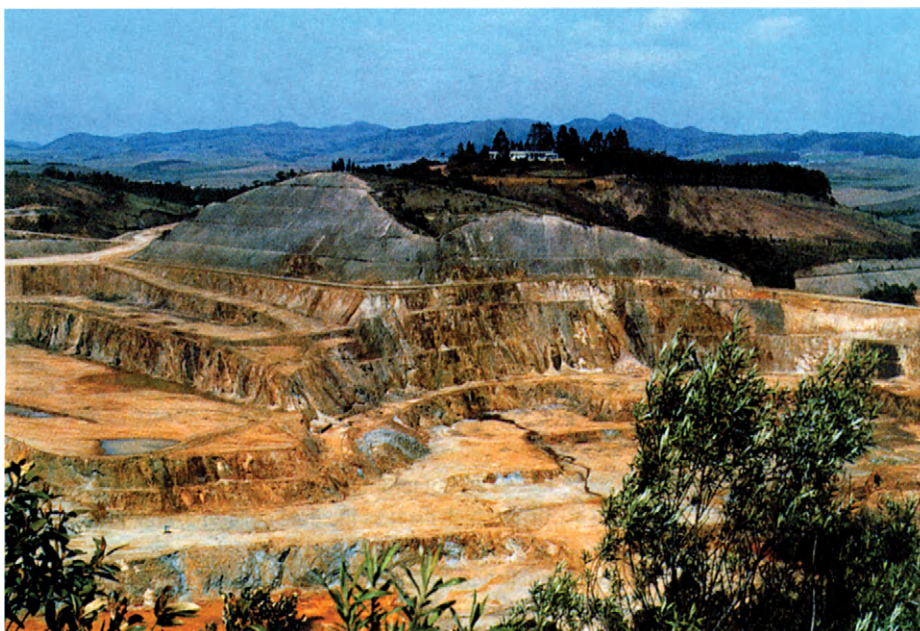
Figure B14.2: Photograph of the Osamu Utsumi mine, showing the redox fronts which were the focus of much investigation. Photograph courtesy of Nagra.
