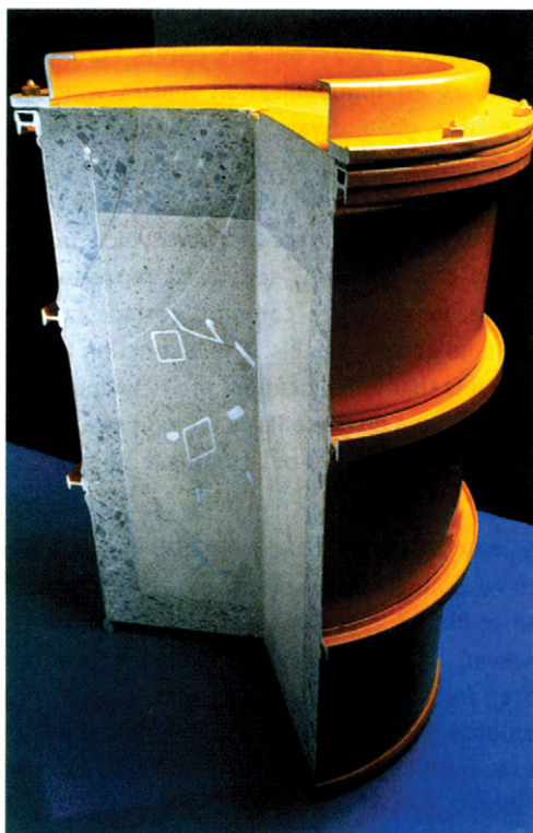
Figure 2.2: Most ILW and LLW will be immobilised in a cement matrix, as shown here in a demonstration waste drum. Several drums may be placed in larger reinforced concrete boxes to create a stable waste package which can be stacked in the disposal vaults in the repository.
