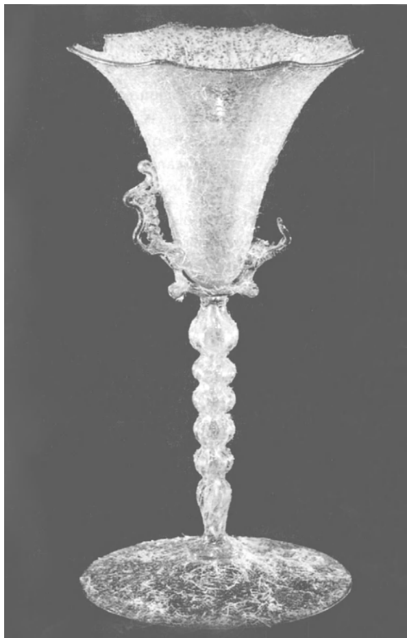
Figure 4.5: An example of extensive crizzling on a Venetian goblet from the collection at the Victoria and Albert Museum in London. Photographs courtesy of Dr. David McPhail.
