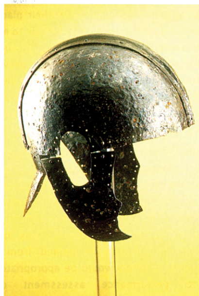
Figure 4.10: Pitting or localised corrosion seen on a Saxon iron helmet. Pitting on a steel canister can cause small perforations to form, allowing radionuclides to escape, before the canister fails mechanically.
