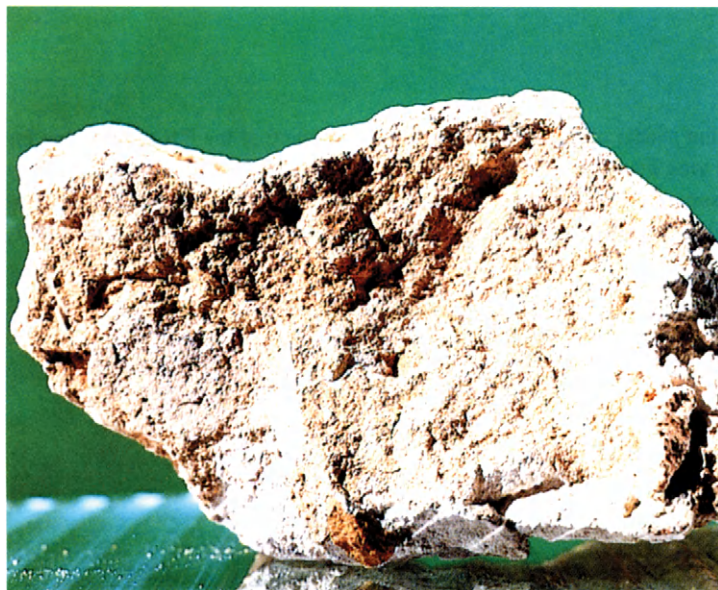
Figure 4.23: Photograph of a section of 1700 year old cementitious mortar from Hadrian's Wall. This mortar contains the same calcium silicate hydrate phases which characterise modern Portland cement.
